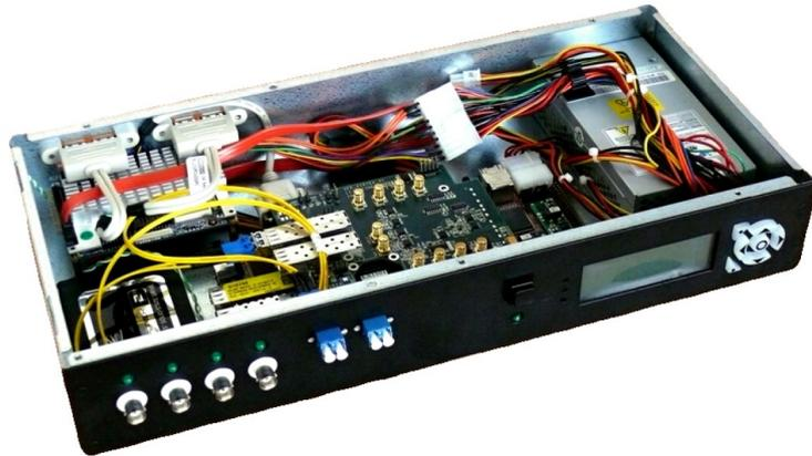
Fig. 3.3: Photo of the time transfer adapter developed by CESNET
