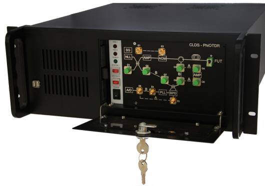
Fig. 3.6: Photo of the own designed and developed DAS.
